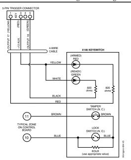
Figure 10. Keyswitch Wiring Connections
